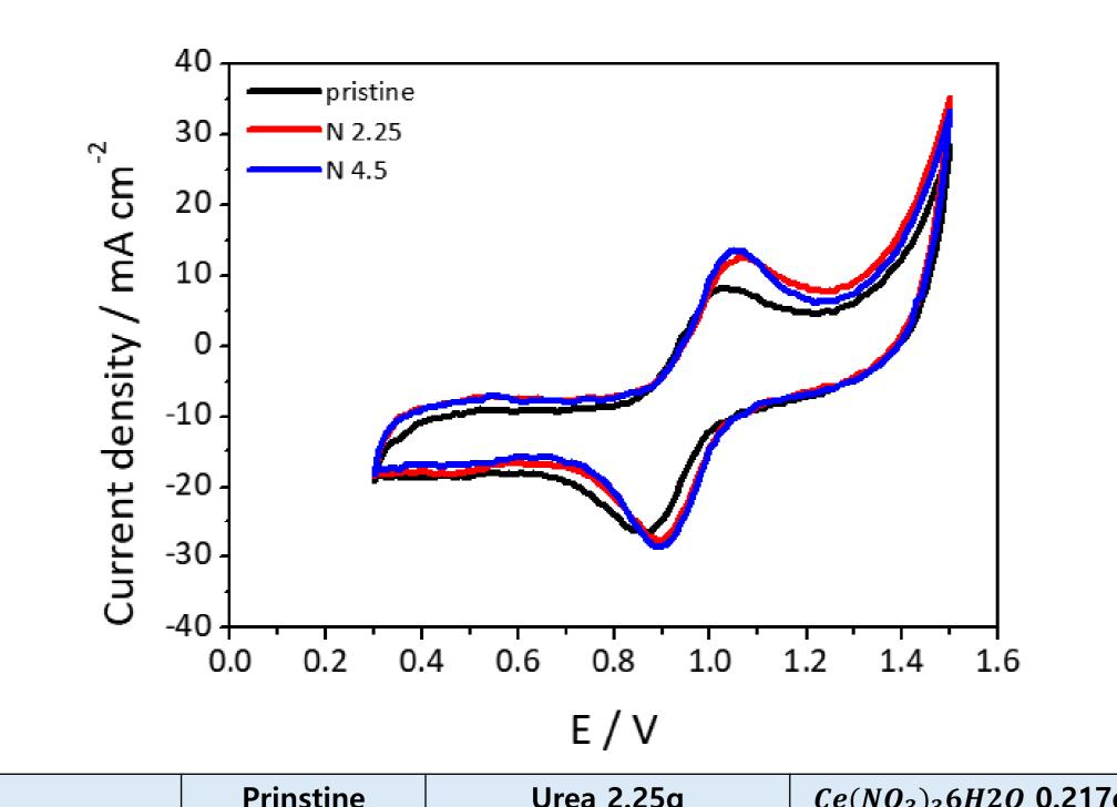
• CV graph according to the N change in carbon paper using  $Ce(NO_3)_3 6H2O$  0.217g
